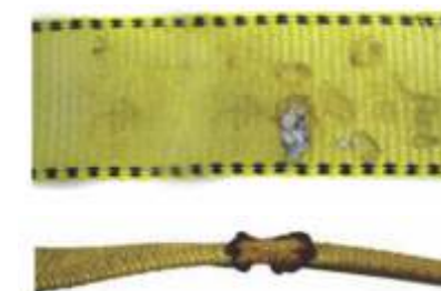
Sling Weld Splatters and Charring/Melting
