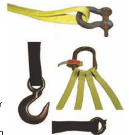
Damaged or Pitted Fittings
