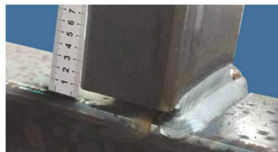
Mild steel / fillet Thickness 2mm, current 110A Unified voltage Clearance 3mm, welding speed 50cm/min
